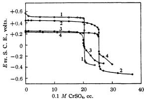
Fig. 1.—Titration of +4 selenium in hydrochloric acid media: (1) 9 N acid at 70°; (2) 6 N acid at 25°; (3) 0.1 N acid at 25°; (4) 1 N acid at 25°.
