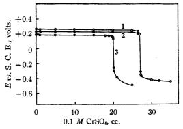
Fig. 2.—Titration of +4 tellurium: (1) 0.3 and 1 N hydrochloric acid, and 1 and 6 N sulfuric acid, at  $25^{\circ}$ ; (2) 6 N hydrochloric acid at  $25^{\circ}$ ; (3) 9 N hydrochloric acid at  $70^{\circ}$ .
