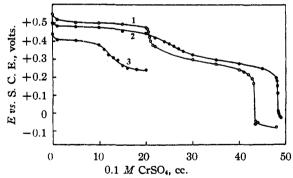
Fig. 4.—Titration of mixtures of +4 selenium and copper: (1) 9 N hydrochloric acid at  $70^{\circ}$ ; (2) 6 N hydrochloric acid at  $25^{\circ}$ ; (3) 6 N sulfuric acid at  $70^{\circ}$ .
